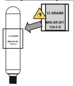
5.1 Check that the size / type of CO2 cylinder is correct for the PFD
